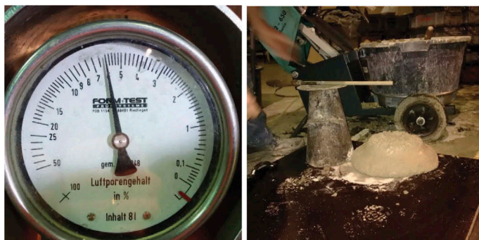
Figure 3. Air content and slump test.
