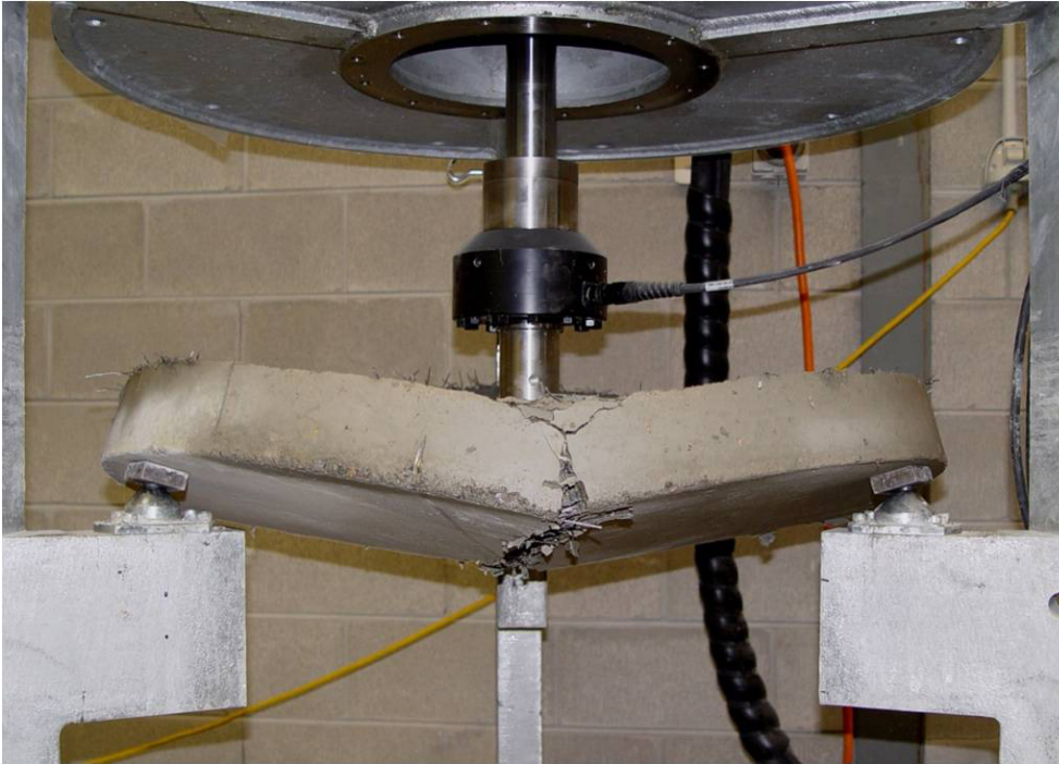
Above: Round panel test. Below: ATSM 1609 beam test
