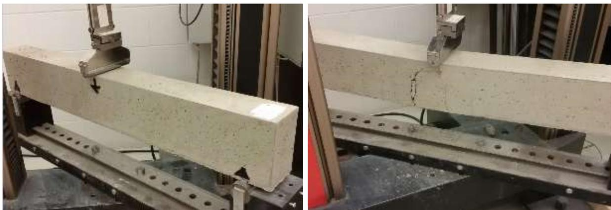
**Pic. 3. Beam before and after testing**
