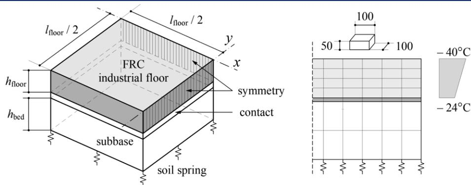
Figure 3: Numerical model (left); mesh and temperature distribution of the numerical model (right)
