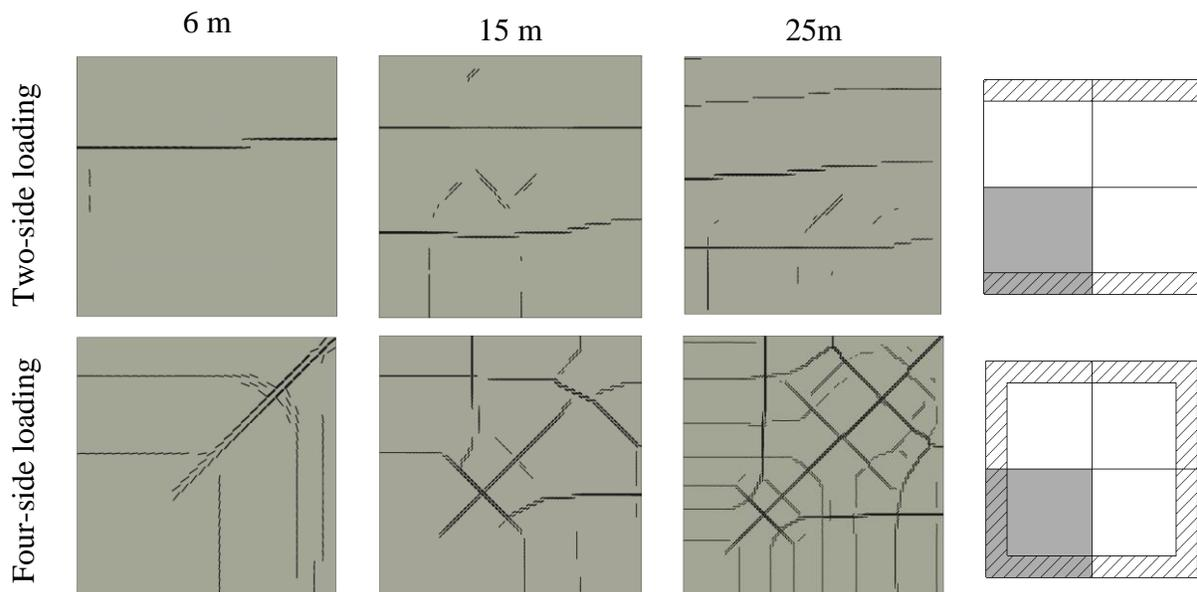
Figure 5: Crack propagation of 2SL and 4SL at 6 m, 15 m, and 25 m, with symmetry condition
