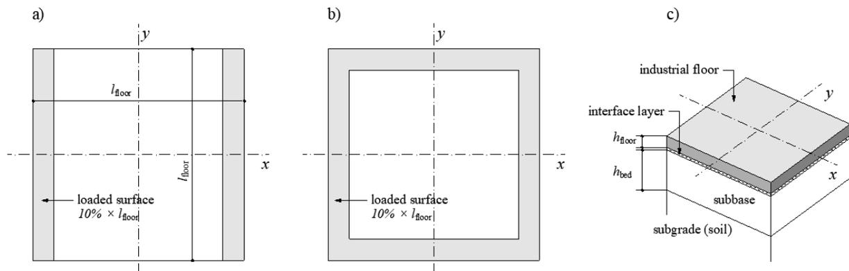
Figure 1: Two-sided load (2SL) (a); four-sided load (4SL) (b); construction of industrial floor (c)
