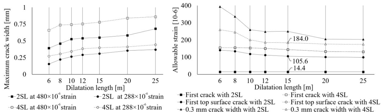
Figure 4: Maximum crack widths (right); allowable strains (left) in the function of dilatation length
