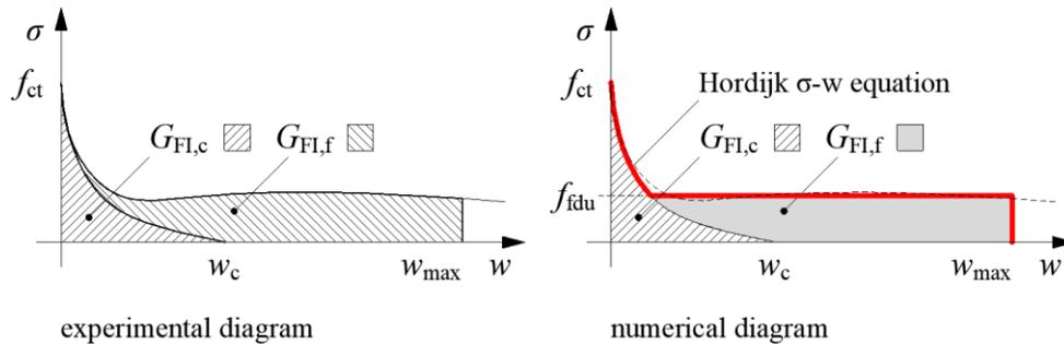
Figure 2: Used material model for fibre reinforced concrete
